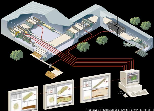
A cutaway illustration of a sawmill showing the Mill Host system analysing data to optimise lumber output at each stage of the mill operation
