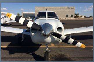
By adding black lines on the propellers, concentric circles are visible when propellers are in motion.
